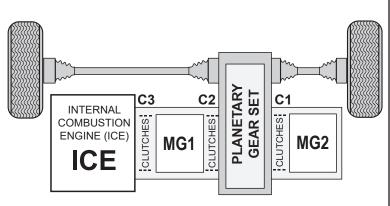
The **Type-4** hybrid-drive is a type of parallel system design.
