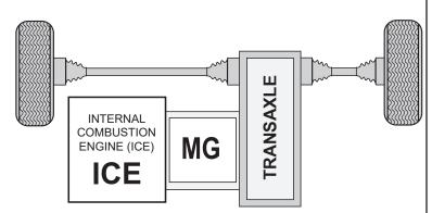
The **Type-3** hybrid-drive system is an extended range electric vehicle which can operate in:
