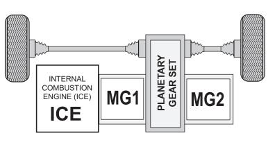
The **Type-2** hybrid-drive is a type of parallel system design.
