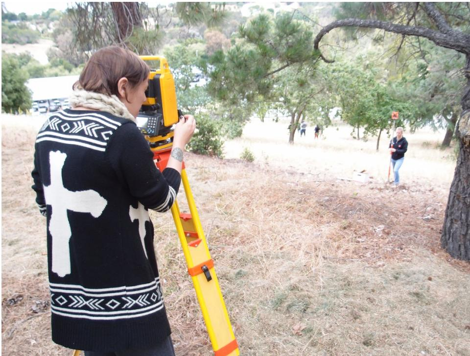
*Figure 2 Students plotting the position of items found with a Laser Total Station during a mock crime scene exercise.*
