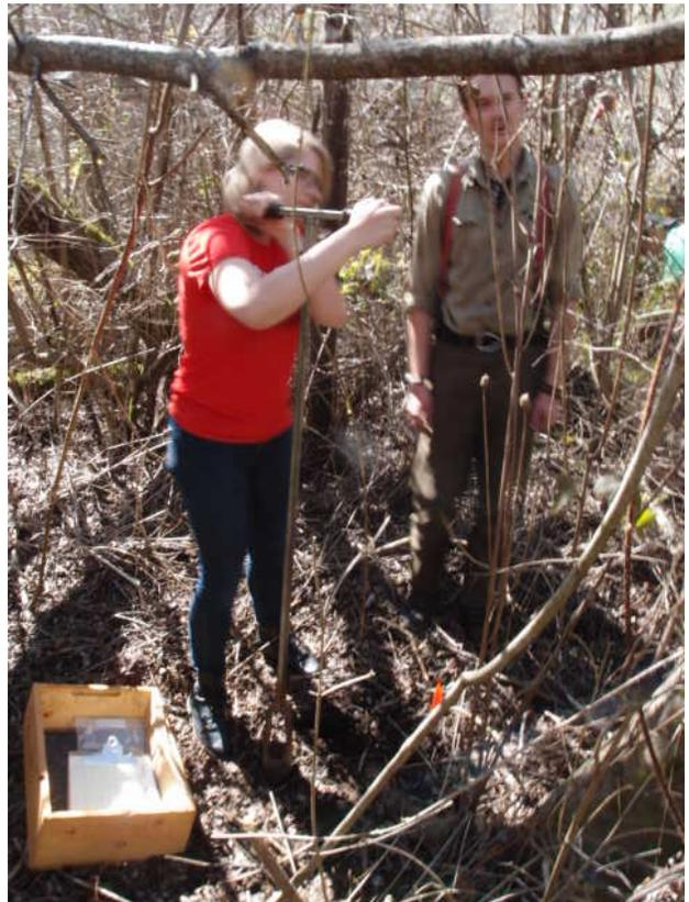
*Figure 5 above is a student using a twist auger to remove a soil core sample for screening, color, and composition testing.*
