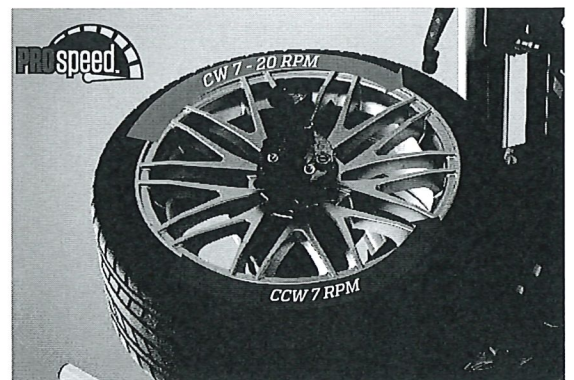
PROspeed™ continuously monitors torque and automatically reduces speed during critical procedures.
