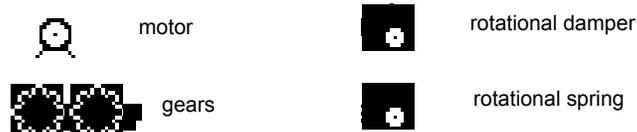
If a rotational constraint is drawn over a single mass object it will attach the mass object to the background beneath (behind) it. If a rotational constraint is drawn over two (overlapping) mass objects, it will attach to both objects.
