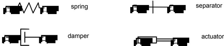
Forces produced by these constraints act equally and in opposite directions upon the mass objects at either endpoint.
