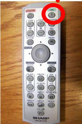
Point this remote at the projector hanging from the ceiling and press the “ON” button. You should hear the fan come on. It will take a minute or two for the unit to warm up.
